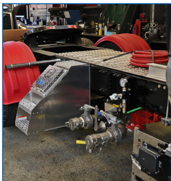
Flow Control System Mounted on Tank or Truck to connect to PTO (drive-line or hydraulically)
